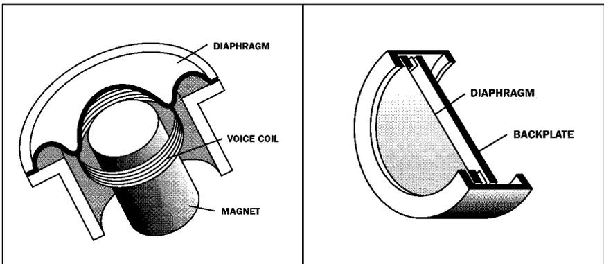
*Cutaway view of dynamic (left) and condenser microphone cartridges*
