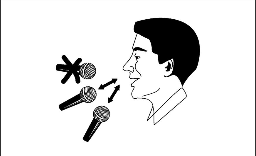
*Illustration: Ideally, a handheld microphone should be positioned six to twelve inches from the user’s mouth, at an angle of 45 degrees or less.*
