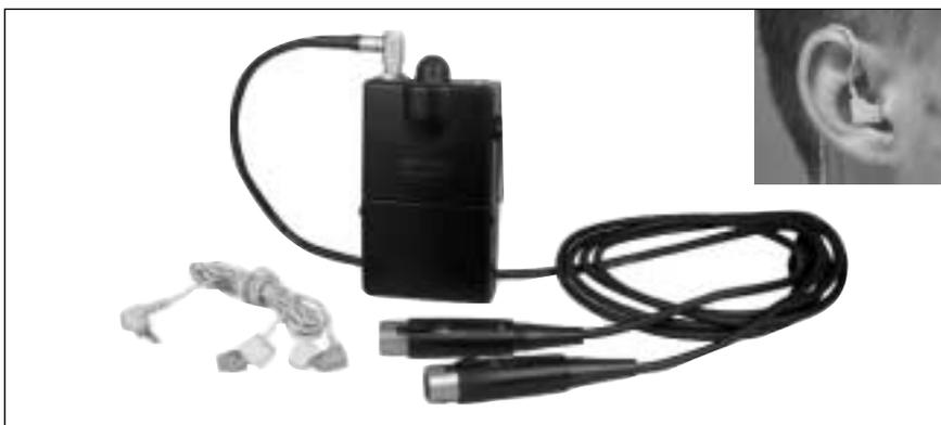
*Example of a Personal Stereo Monitoring (PSM) System
